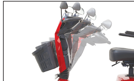
Infinite adjustable tiller with ergonomic design
